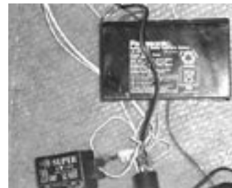
Above: Panasonic 7 Ah battery with solar regulator, recommended to prevent the battery from overcharging, and shortening its life.
